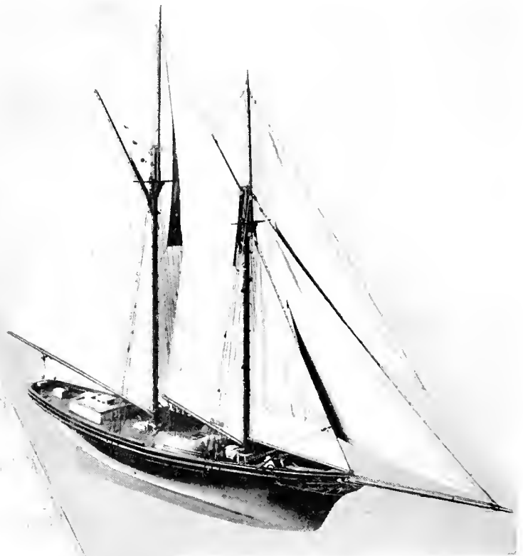
FISHING SCHOONER Fredonia , rigged model USNM 160211. This vessel, designed by Edward Burgess and built in 1889, influenced the design of New England fishing schooners for about fifteen years. (Smithsonian photos: Top, 44956-b; and bottom, 44956-c.)
